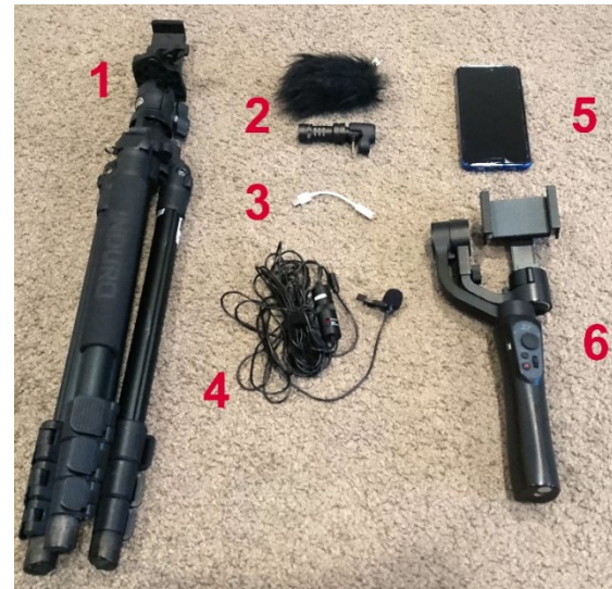
Figure 1. Image illustrating the hardware used by the author. (1) Induro tripod. (2) Rode VideoMic Me with “deadcat”. (3) USB-Type C adaptor (4) Boya lavalier microphone (5) Huawei P20 smartphone (6) Zhiyun Smooth-Q gimbal.
